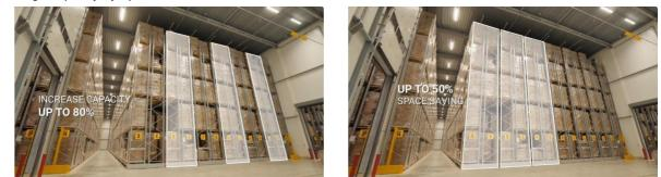
2, Accessibility: The movable shelving units allow for easy access to stored items, as the aisles can be opened only when needed.
